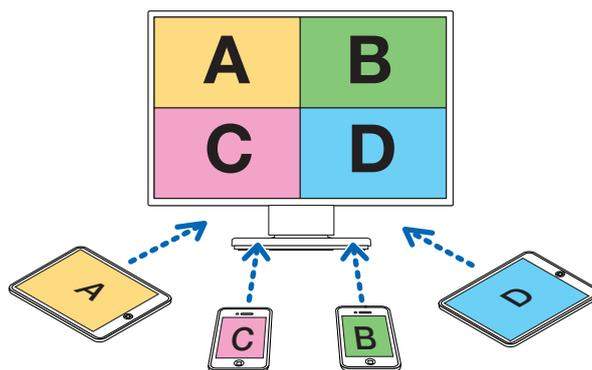
● **Simultaneous Display onto multiple receiving devices**
